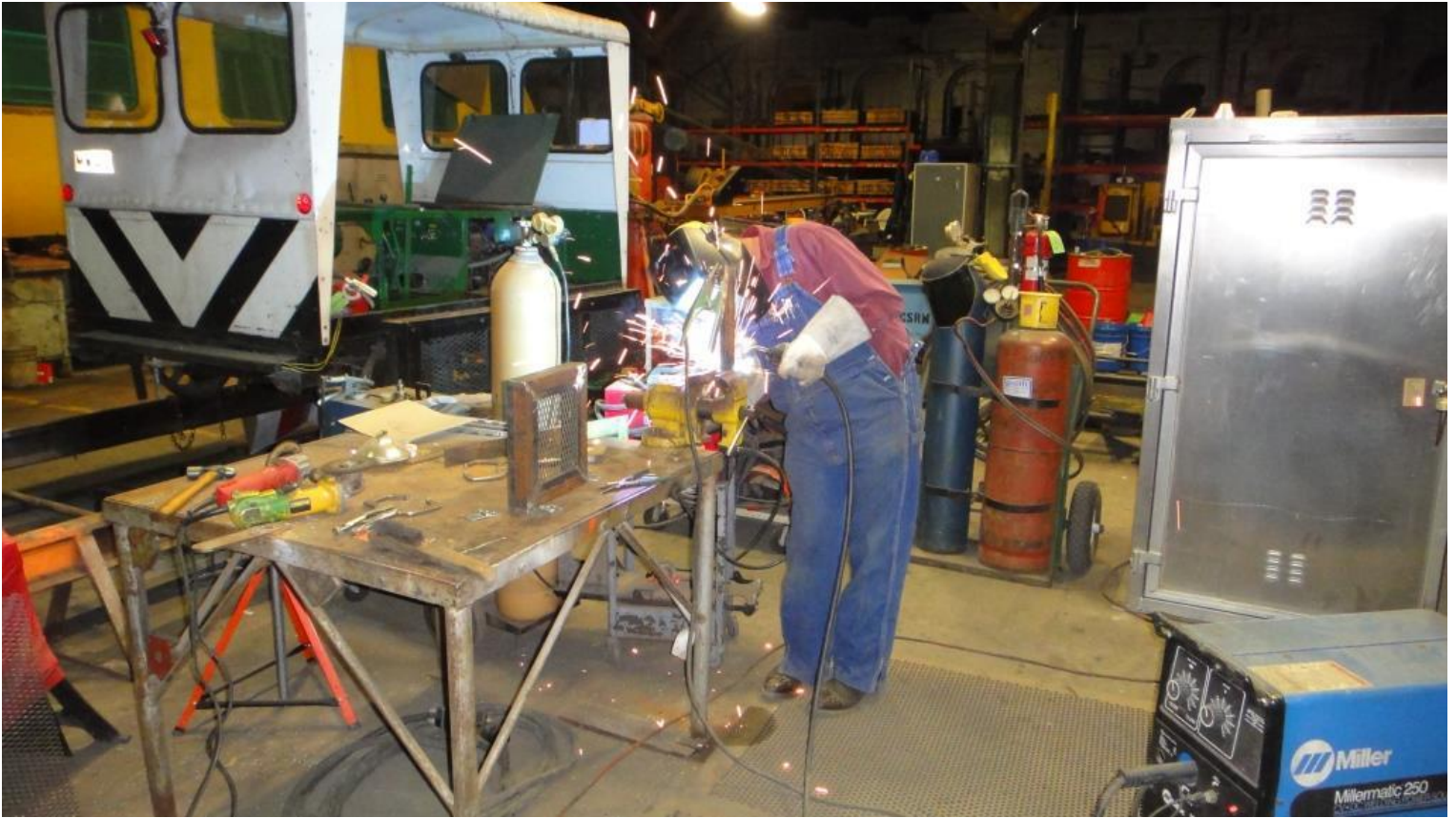
Cliff building a protective cage for the turntable controls on the ballast regulator
